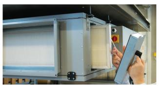
> Filter change. Filter pollution is monitored by pressure switches or a timer. Filters are easily removable: in the CXP series there's even no need to remove the cover. This is critical when the unit hangs under the ceiling.
