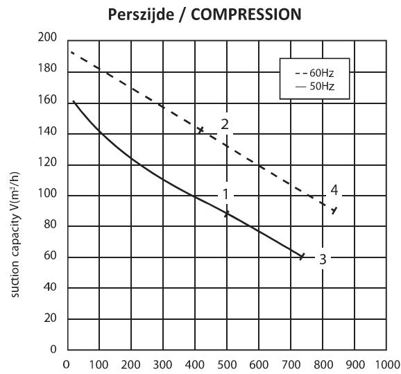
The characteristic data given here refer to the handling of gas with inlet temperature of 15° C, normal density of 1,23 kg/m³ and absolute pressure of 1.013 mbar. Tolerance of ±10%. The data may change without any notification.
