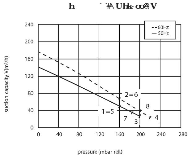
The characteristic data given here refer to the handling of gas with inlet temperature of 15° C, normal density of 1,23 kg/m<sup>3</sup> and absolute pressure of 1.013 mbar. Tolerance of ±10%. The data may change without any notification.
