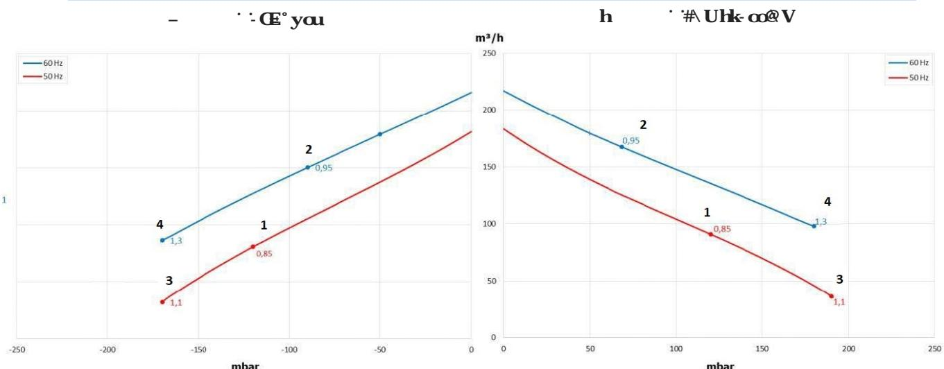
The characteristic data given here refer to the handling of gas with inlet temperature of 15° C, normal density of 1,23 kg/m<sup>3</sup> and absolute pressure of 1.013 mbar. Tollerance of ±10%. The data may change without any notification.
