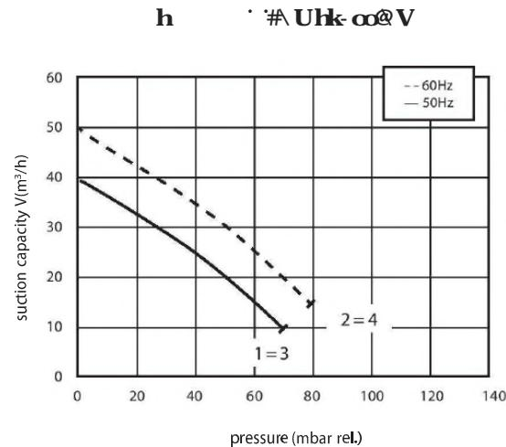
The characteristic data given here refer to the handling of gas with inlet temperature of 15° C, normal density of 1,23 kg/m³ and absolute pressure of 1.013 mbar. Tollerance of ±10%. The data may change without any notification.
