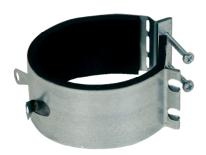
These fast clamps facilitate with the installation and removal of fans for service and cleaning. The extra holes make it easy to install the fan in a canal. The fast clamps are made from galvanised sheet steel and fitted wth an 8 mm neoprene lining which suppresses vibrations and ensures a tight fit.
